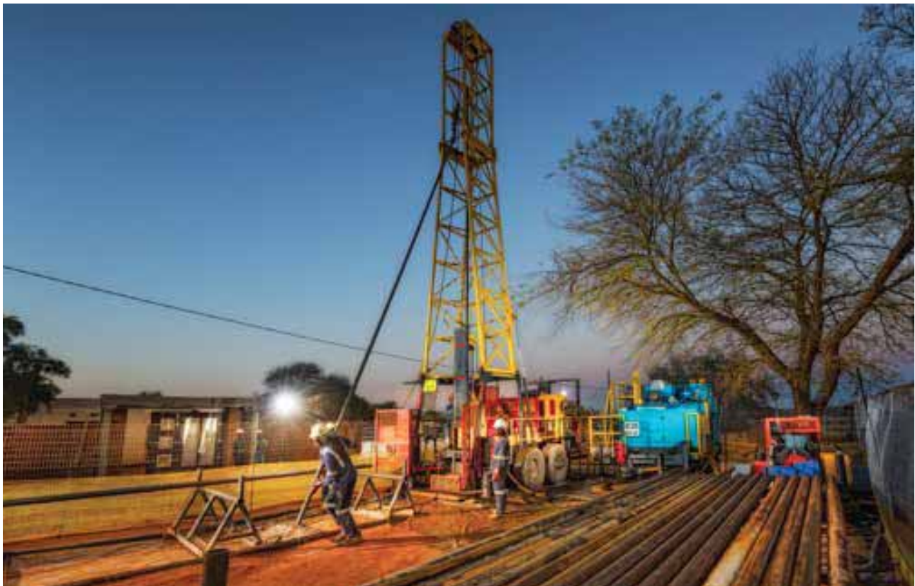
Exploration drilling, BRPM North shaft Phase III investment area
