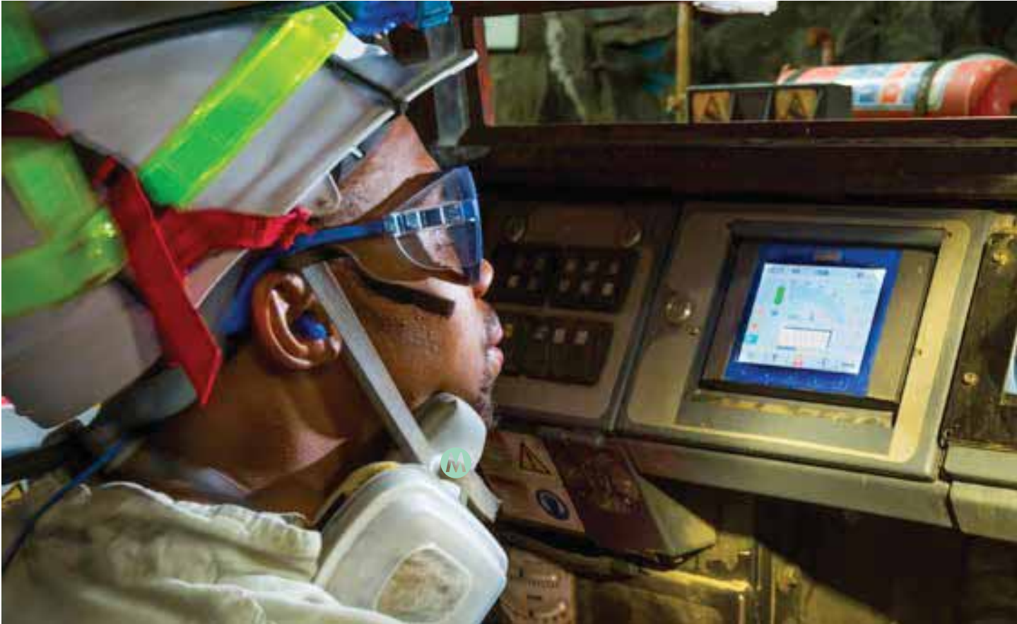
The infrared cameras providing the driver of an LHD in Styldrift I mine with a view of what are normally blind spots
